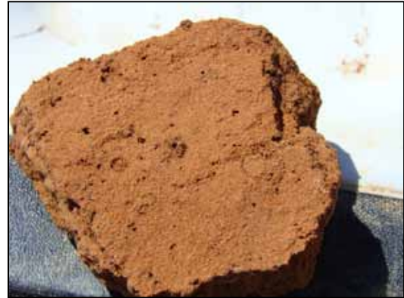
Figure 7-2 Pinholes in collapsible soil (courtesy of Brian Moffat, NRCS Texas State geologist)
