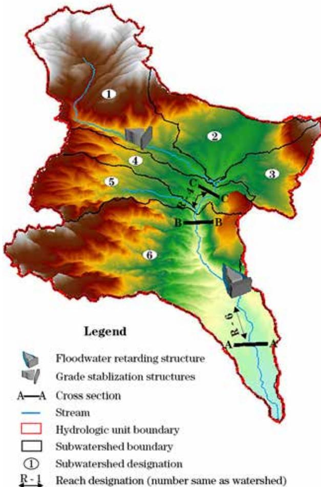
In selecting reaches, the method of computing water surface profiles may specify a maximum or a minimum length of reach. Some hydraulic models, such as HEC-RAS have a user defined capability to interpolate sections as specified intervals between specified sections or along an entire reach. However, even these programs have limitations that must be observed.
