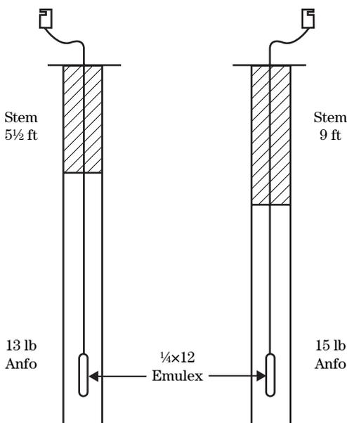
**Figure 7-10** Presplitting in the bypass and auxiliary spillway at Hughes River Dam in West Virginia
