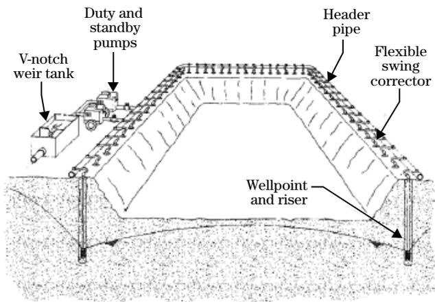
Inspectors must verify that groundwater control systems are functioning properly. A system that is not functioning properly can often be detected in early stages by visual observation of:
