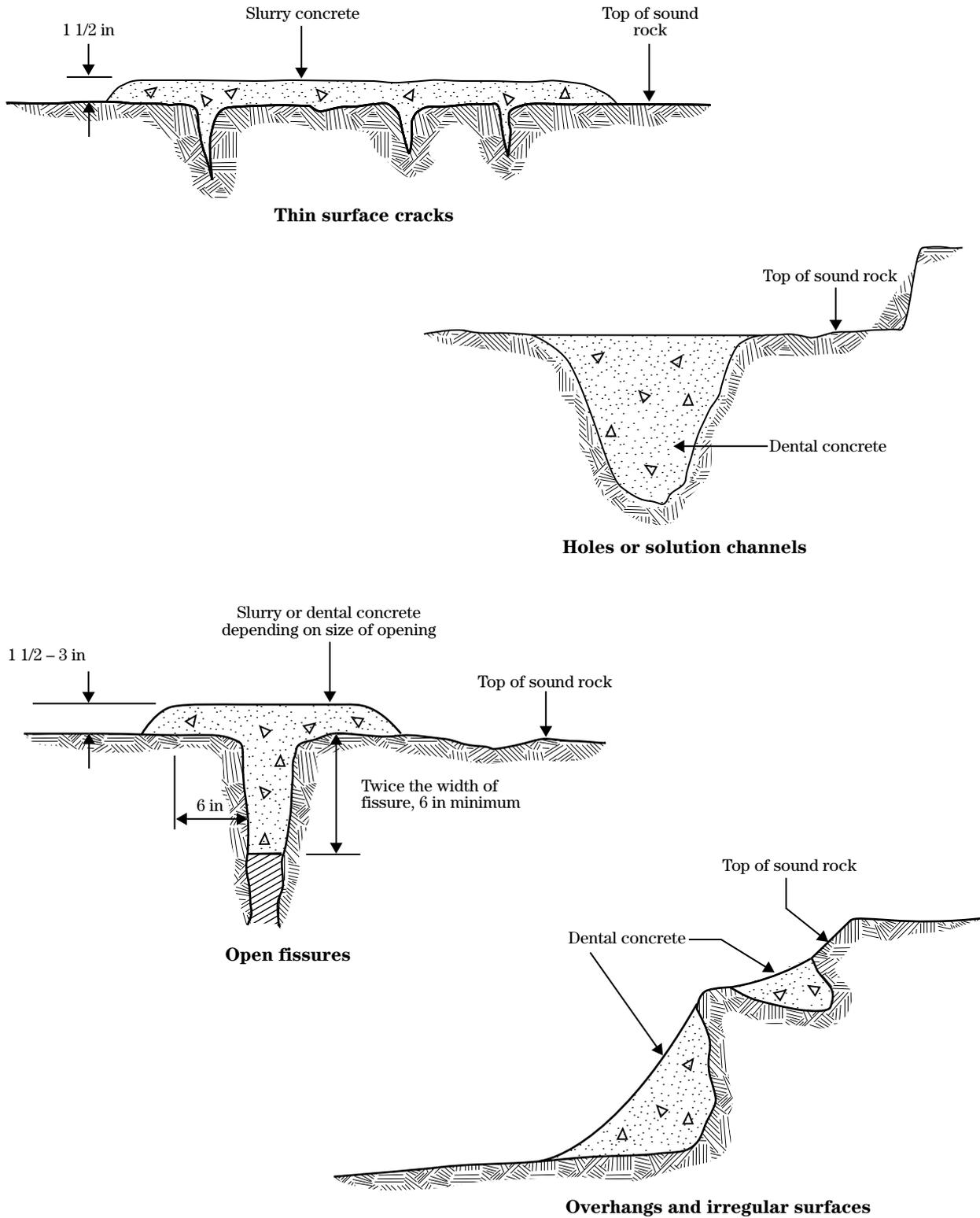
to see that changes from the expected design conditions are documented and reported to the responsible engineer. Undesirable conditions in rock foundations may include zones of weathered or fractured rock; cavities; soft soil areas; abandoned pipes or drains; or abandoned stream channels filled with clay, silt, sand, or gravel.
