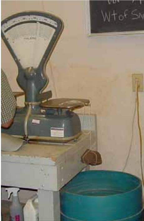
*Step 4* Weigh wax-coated clod submerged in water.
