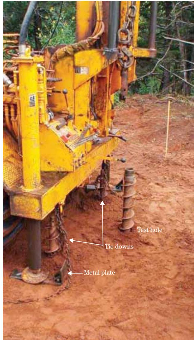
**Figure 11-7** SCPT being conducted through hollow stem augers (Photo courtesy of Glen Miller, Geologist (retired), NRCS, Stillwater, Oklahoma)
