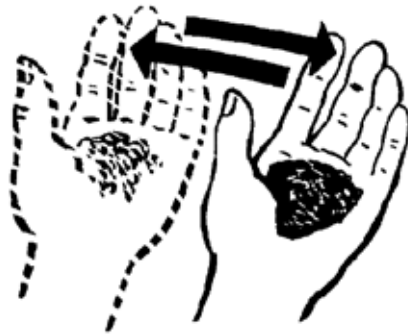
Dilatancy test: Shaking wet soil
