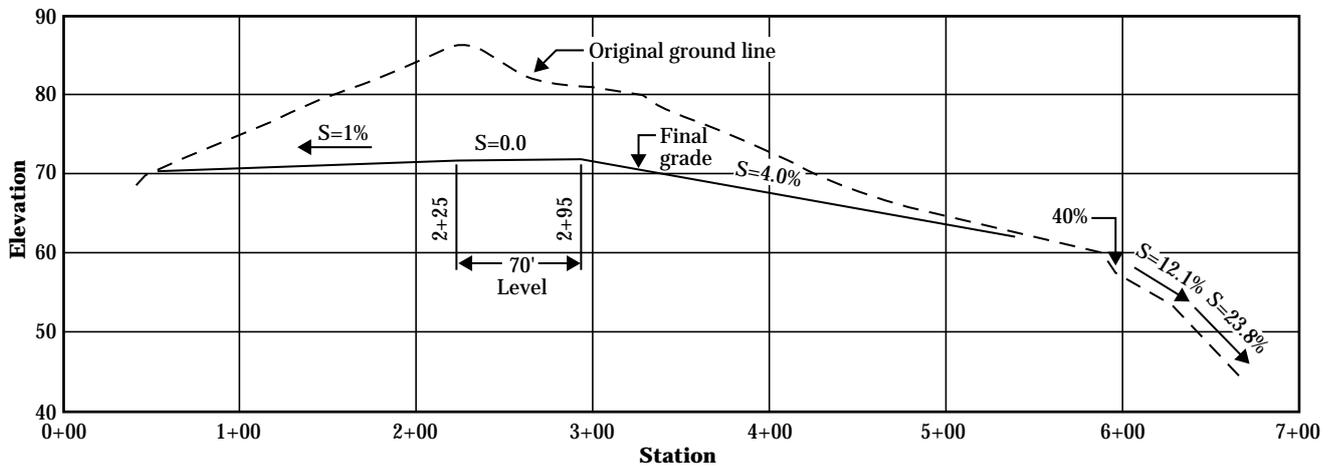
**Figure 50-6** Outlet of spillway exit channel extended to flood plain
