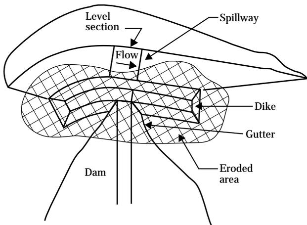
**Figure 50-4** Spillway gully resulting in breach of spillway
