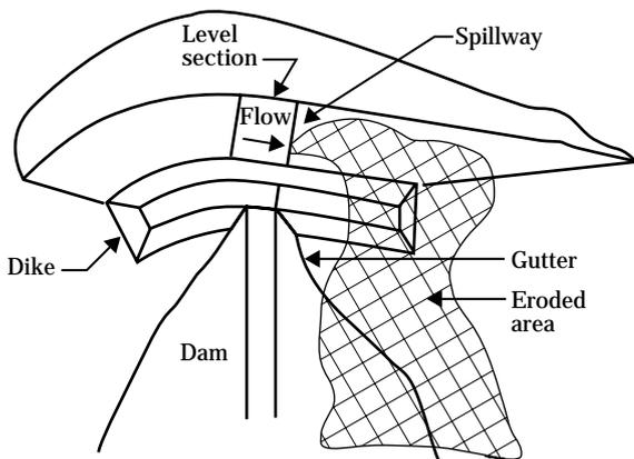
**Figure 50-2** Early failure of retaining dike
