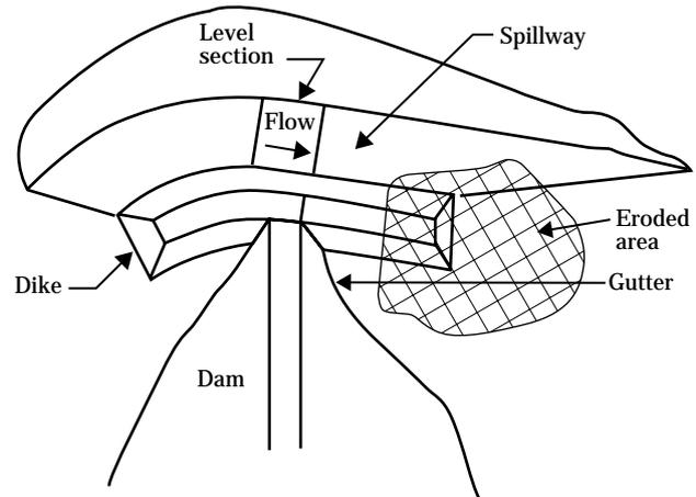
**Figure 50-3** Erosion of spillway and retaining dike resulting in breach of spillway, dike, and dam
