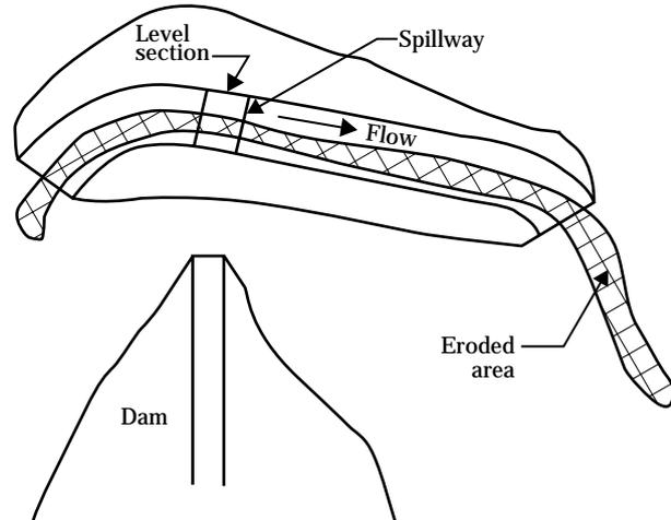
alternate layout could be assessed that uses a uniform grade of about 7 percent from the crest to the flood plain. The alternate layout will increase excavation.
