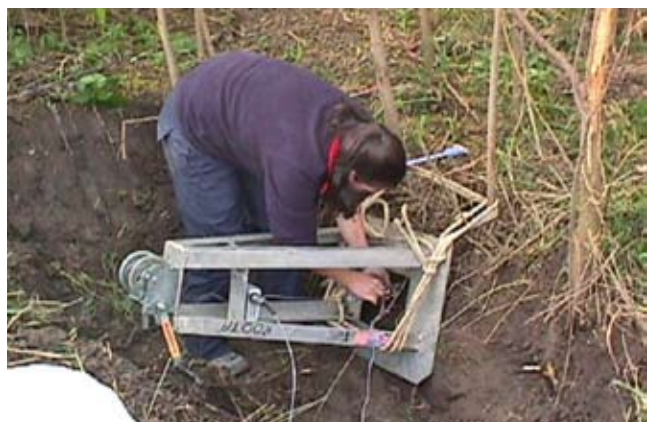
Figure CS9–21 Root strength testing
