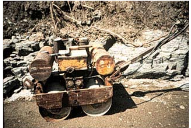
Figure CS4-7 Manually directed vibrating drum roller
