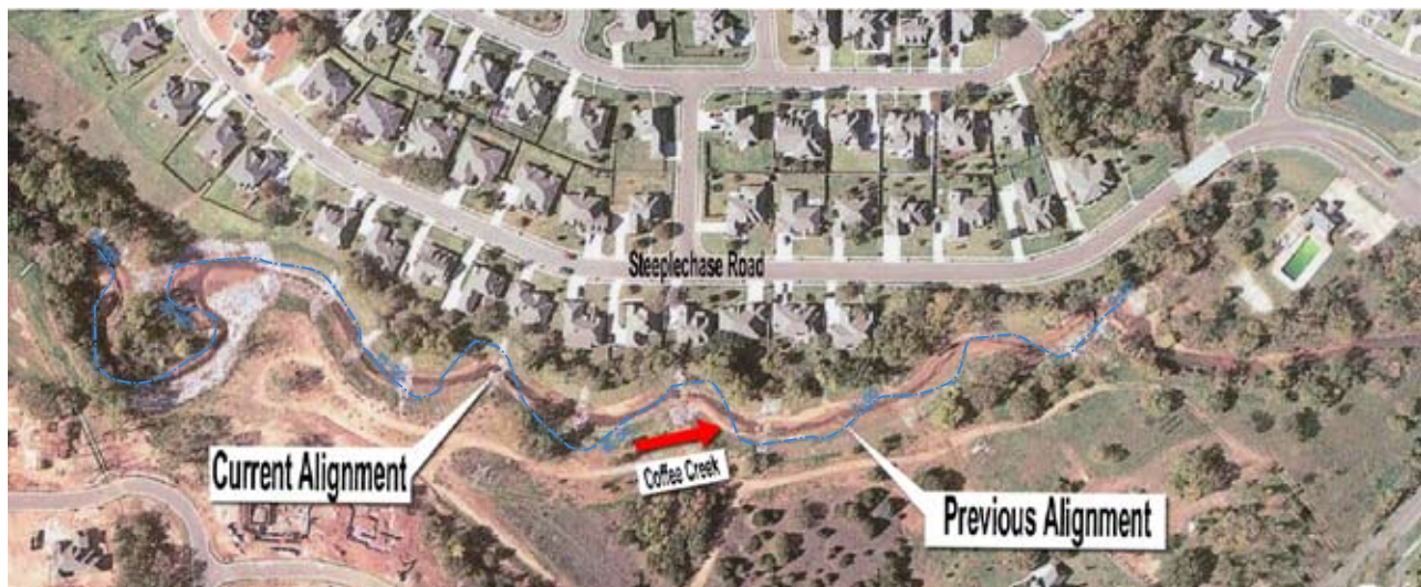
Figure CS16-6 Aerial view of project channel alignments
