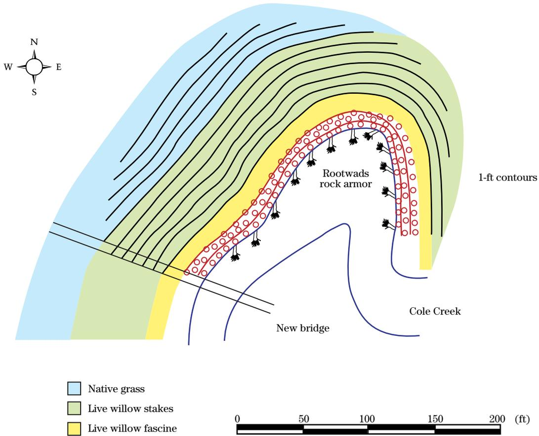
Below the willow stakes, 450 feet of live willow fascine would be installed for additional root mass and flow energy deflection from the slope toe. To maintain access to the fairway, the top of the slope was to be planted with a mix of deep-rooted native grasses, including switchgrass, buffalograss, and big and little bluestem grasses. These grasses would take up more soil moisture with their larger and deeper root network and require little to no additional watering.
