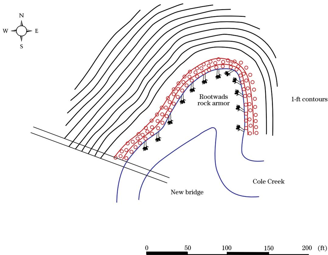
Figure CS11-11 Soil bioengineering and planting plan
