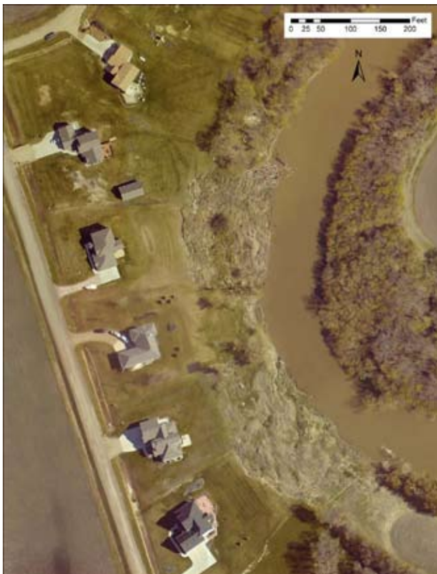
Figure CS11-4 Slump flows caused by septic drain fields near Fargo, ND
