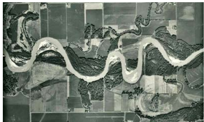
Figure 12–13 Meandering with point bars and chute channels, Type c ( T_c )
