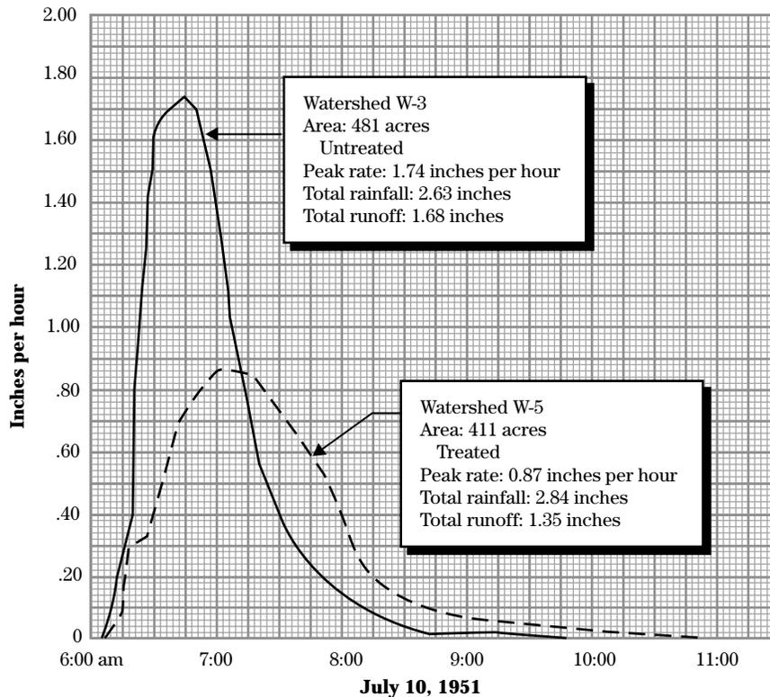
Since  $T_p$  consists of storm duration and time of concentration (see NEH 630, chapter 16), the changes in either (or both) factors can be studied in a graph similar to that of figure 12-4. The graph shows that, for this case, the second type of lag effect becomes relatively insignificant at about  $T_p = 5$  hours.
