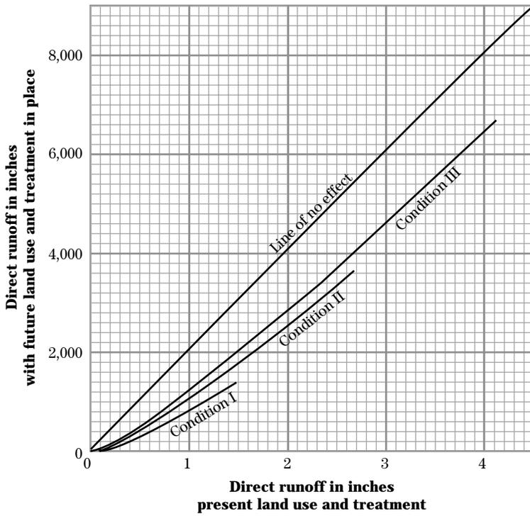
Quite often the first type of lag (producing increased infiltration) can be assumed to take place in the manner of the second type of lag which causes a delay in surface runoff arrival. The technique that follows can be used to estimate expected changes in hydrograph quantities.
