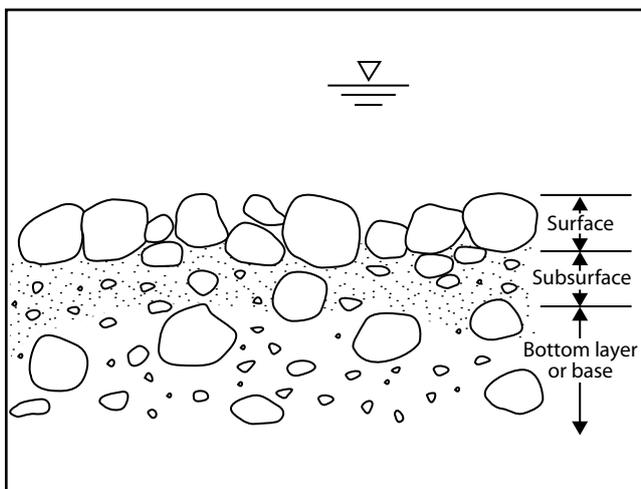
**Figure TS13A-4** Coarse bed stream sampling hierarchy
