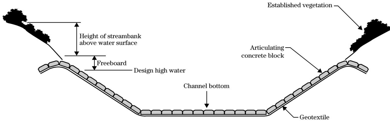
**Figure TS14L-2** Armoring the toe and lower slope cross section
