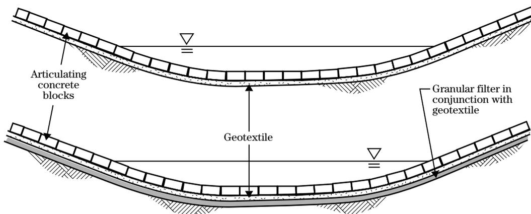
**Figure TS14L-11** ACBs in combination with granular and geotextile filter
