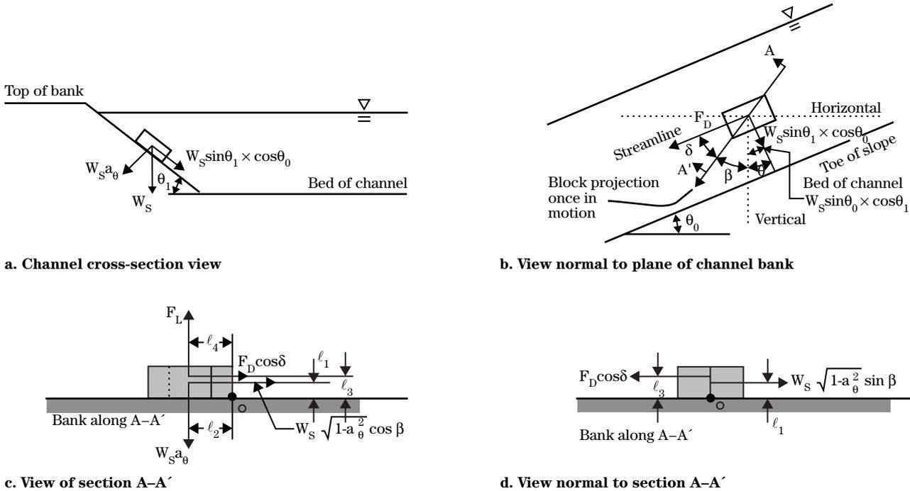
**Figure TS14L-16** Block moment arms (*Figure courtesy of HCFCD*)
