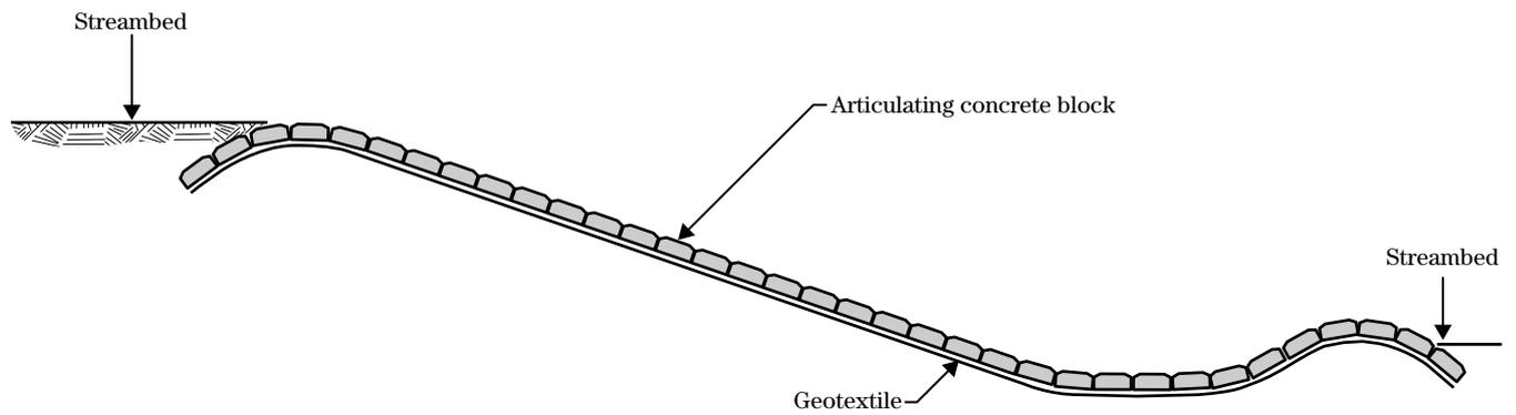
**Figure TS14L-5** Armoring of pipe/culvert outlets profile
