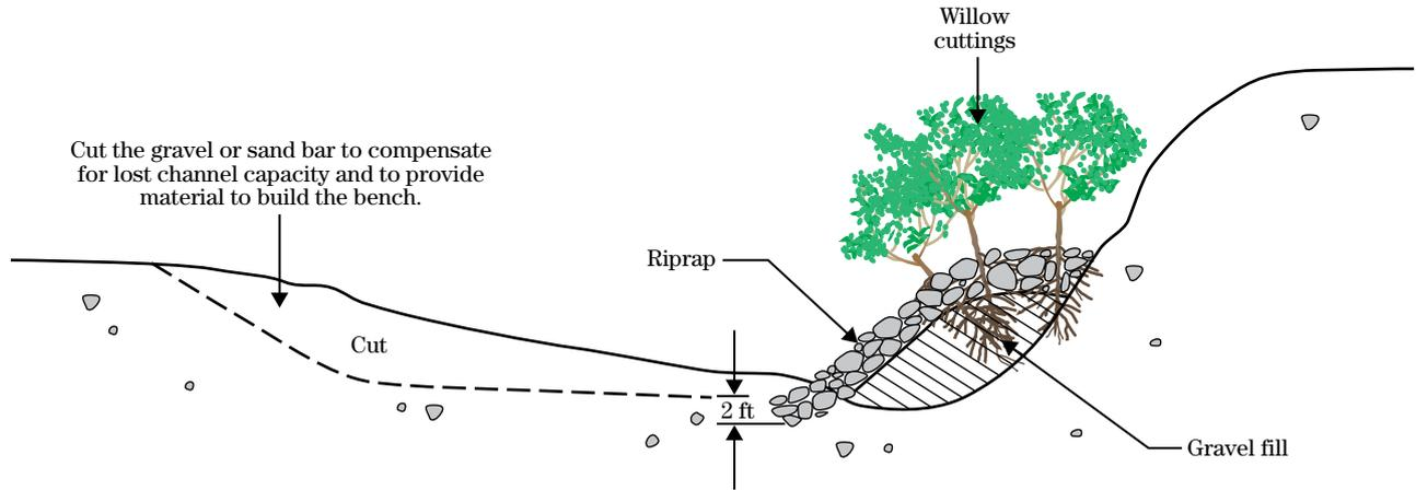
**Figure TS14K-4** Excavated bench method
