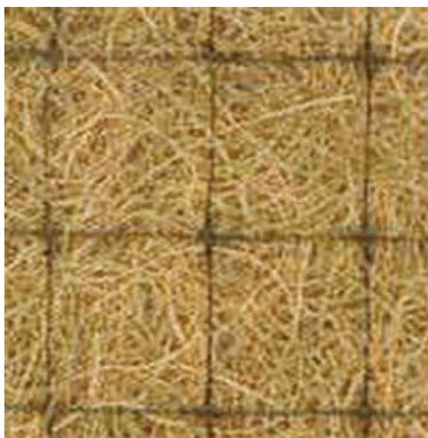
**Figure TS14D-9** Turf reinforcement mats
