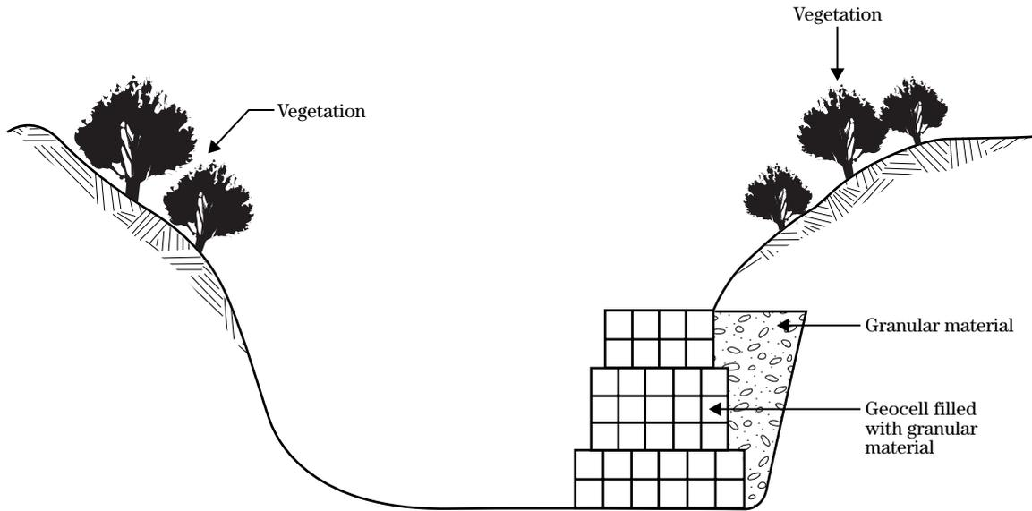
**Figure TS14D-14** Erosion protection
