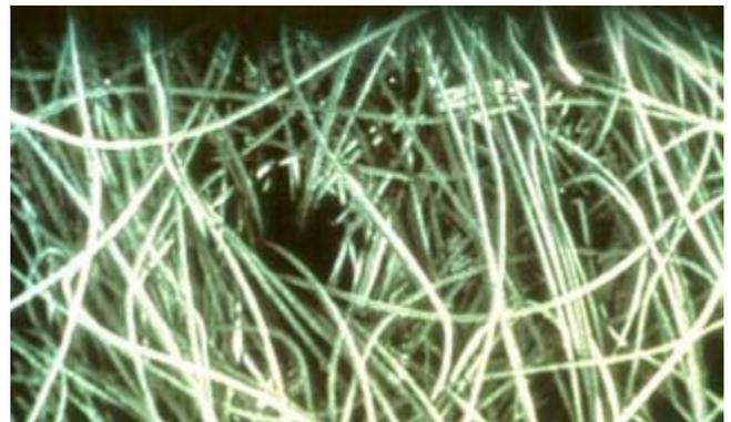
**Figure TS14D-3** Heat-bonded nonwoven geotextile
