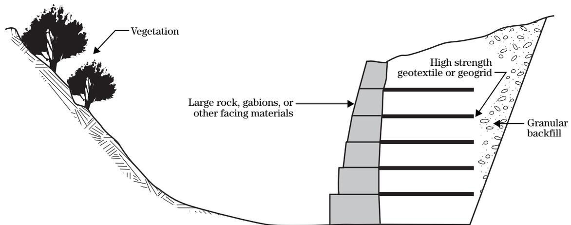
**Figure TS14D-13** Earth retaining structure
