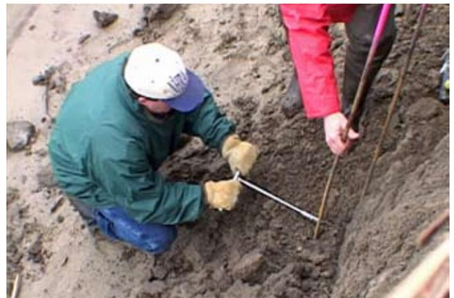
**Figure CS9-17** Installing bank erosion pins
