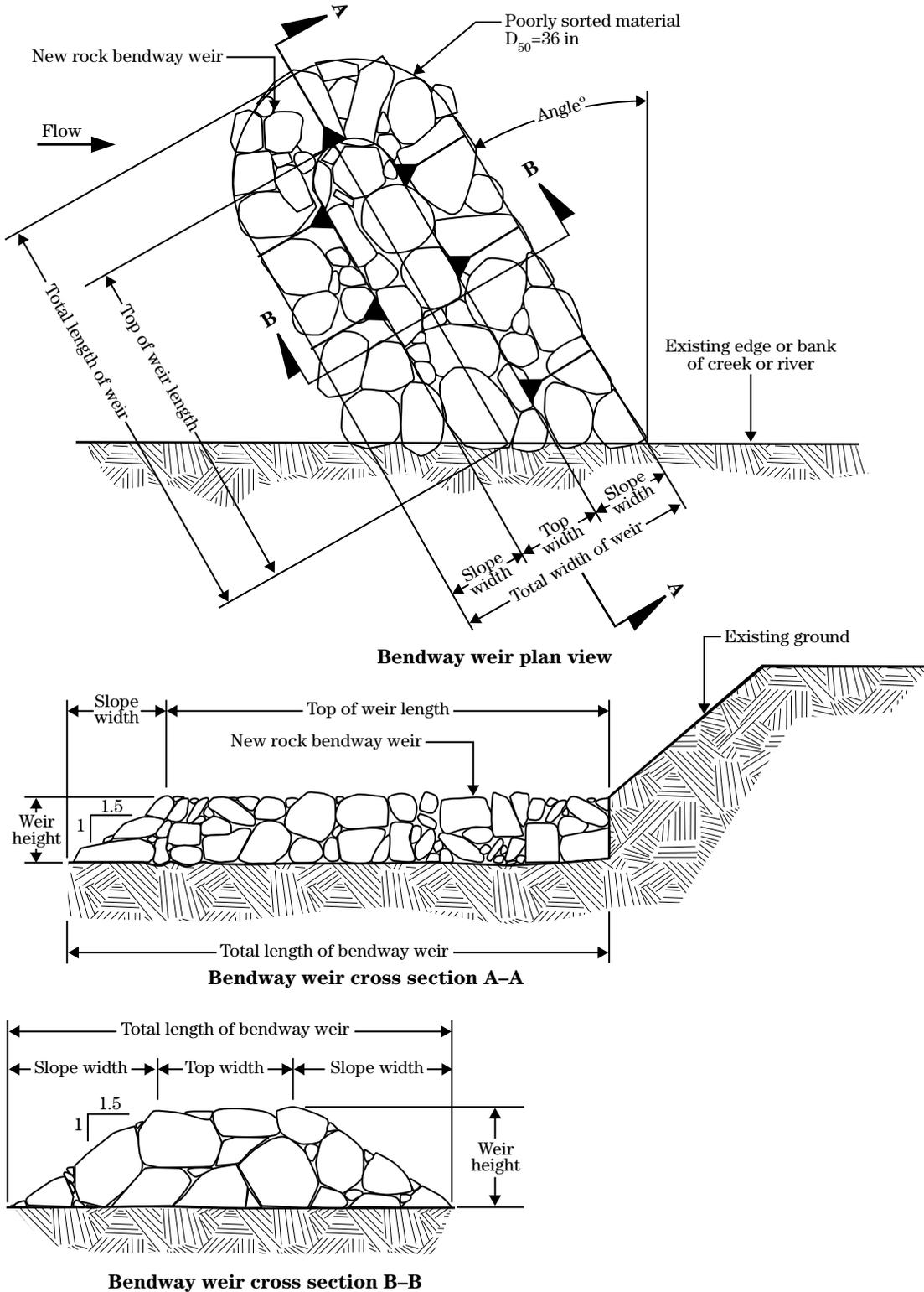
Figure CS9-5 Rock vane design detail
