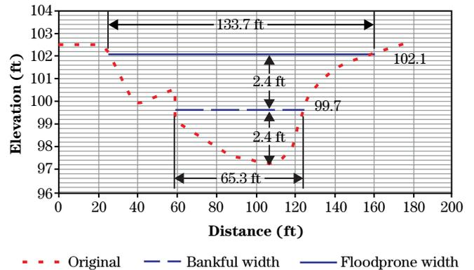
**Figure CS3-7** Cross section of undisturbed site upstream
