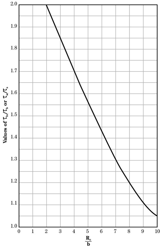
**Figure 8-9** Applied maximum applied shear stress,  $\tau_{bt}$  and  $\tau_{st}$  on bed and sides of trapezoidal channels in straight reaches immediately downstream from curved reaches
