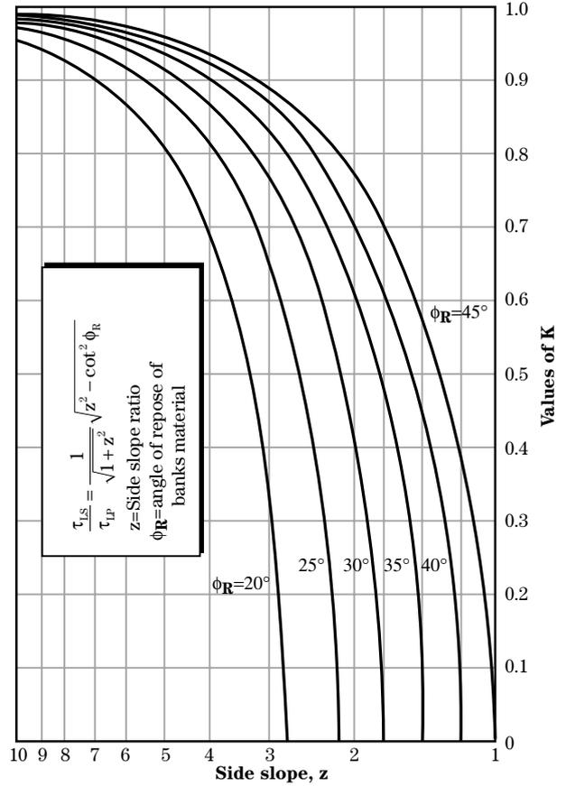
**Figure 8-16** Allowable shear stress for granular material in straight trapezoidal channels
