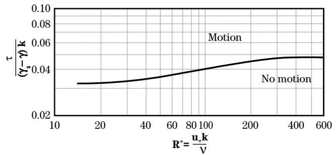
**Figure 8-10** Shields curve
