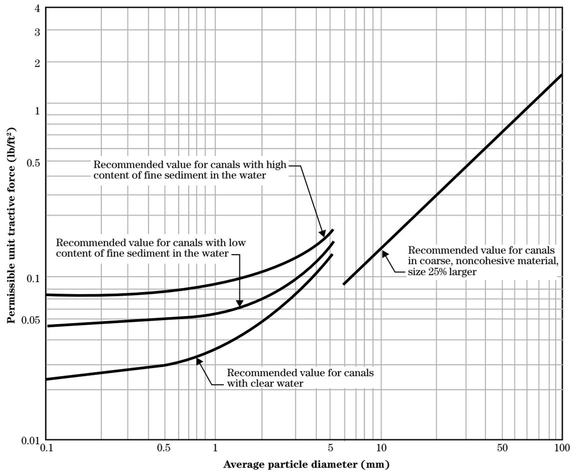
**Figure 8-17** Allowable shear stress in cohesive material in straight trapezoidal channels
