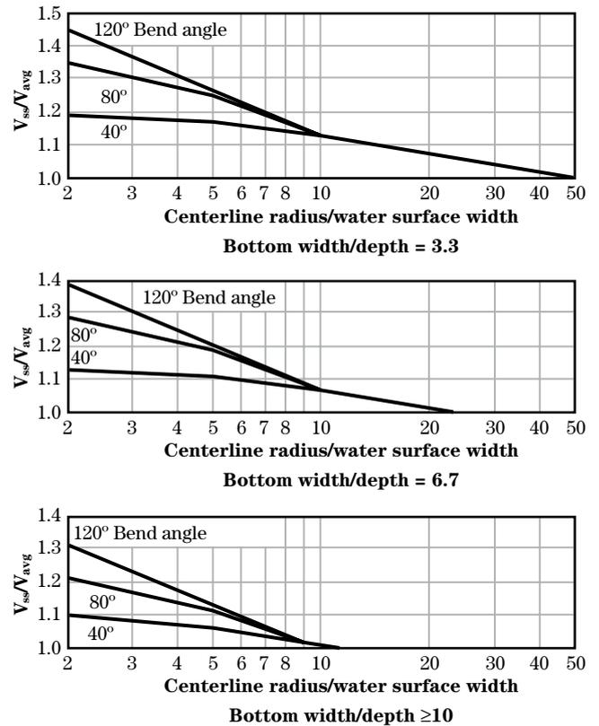
Notes:  $V_{ss}$  is depth-averaged velocity at 20% of slope length up from toe, maximum value in bend. Curves based on STREMR model (Bernard 1993),  $V_{avg} = 6$  ft/s, 1V:3H side slopes.  $n = 0.038$ , 15 ft depth
