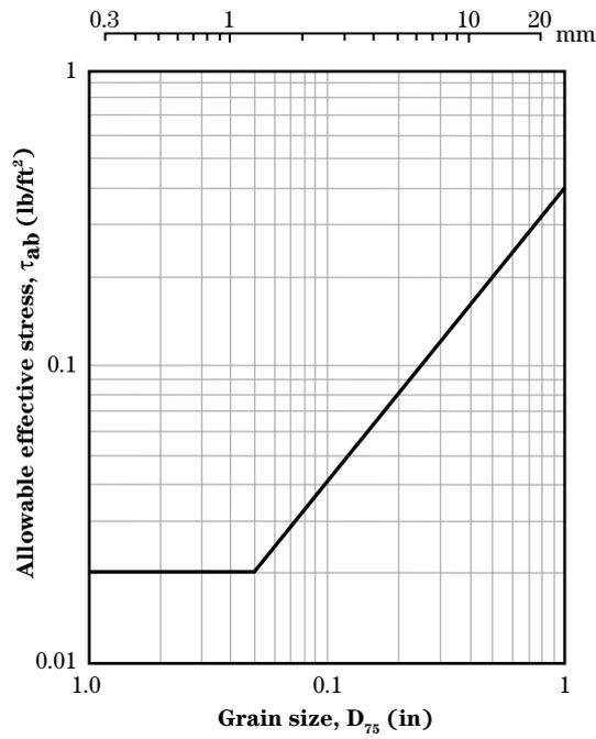
**Figure 8-22** Soil grain roughness for noncohesive soils
