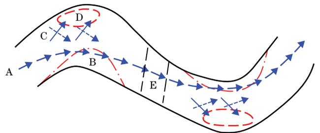
currents angle into the bank and undercurrents move away from the bank, a zone of downwelling results at point D. The low bed load gives the stream a scouring tendency. Toward the inflection point of the meander, flow with a low bed-load supply enters a contracted reach at E that is steeper and shallower, and regains its scouring capacity. Riffles form and, as the highest velocity vectors cut from one point bar toe to the toe of the next downstream bar, riffles are often skewed to the banks.
