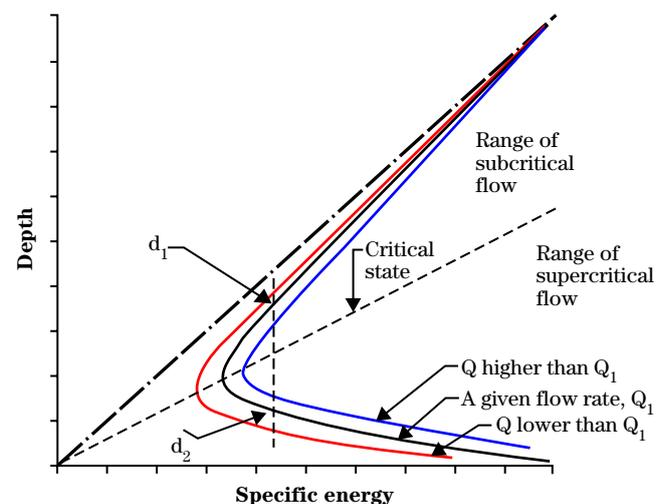
small change in energy results in a relatively significant undulating change in depth. An understanding of flow energy is fundamental in hydraulic modeling.
