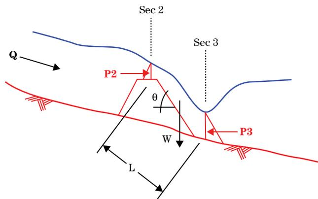
However, the weir will not cause a hydraulic jump if it is drowned out by downstream tailwater. The downstream depth must be less than critical depth over the weir plus the weir height, or, using the definition of critical depth:
